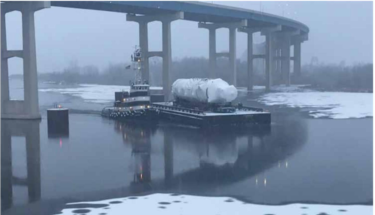
Our new vacuum tower arrived via barge. The 125 foot tall piece was installed on the refinery grounds in late January, an important element in crude processing.
